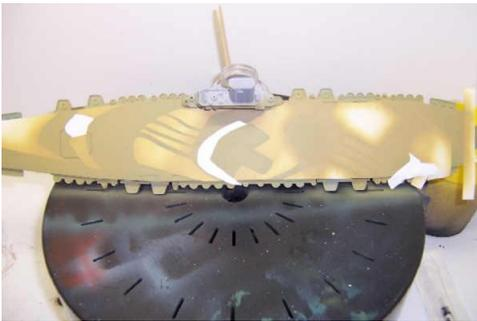
Using the line drawing of the masks, begin placing the pieces of the masks. Make sure each piece is rubbed down thoroughly. If the masks does not completely cover the area, which is a possibility, fill in with either masking tape or pieces of the masking vinyl that you removed.
